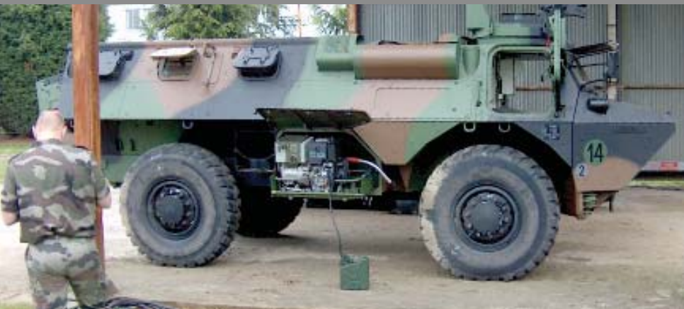
Generating set specifically designed for its application in armored trucks
