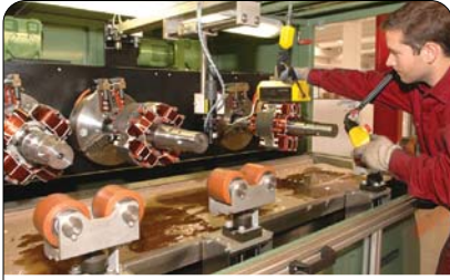
The "DIP and ROLL" impregnation guarantees high resistance to torsion vibrations
