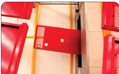
The metals of HIMOINSA offer higher resistance to corrosion thanks to the implementation of a film forming passivating system in the painting stage
