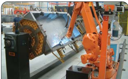
MIG/MAG welding technique for precise finishing and sealed welding beads
